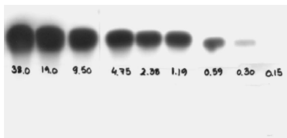
Fig. 1. Autoradiogram of a thin-layer chromatographic plate (Si 60; n -butanol–acetic acid–water, 4:4:1) with applied amounts of chloride from 38.0 to 0.15\ \mu\text{g} . The starting and end lines of the plate are at the bottom and top of the film, respectively. The exposure time was 4 days.
